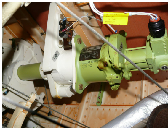
Photo 17. Load Limiter of the main right alternate landing gear extension system.
