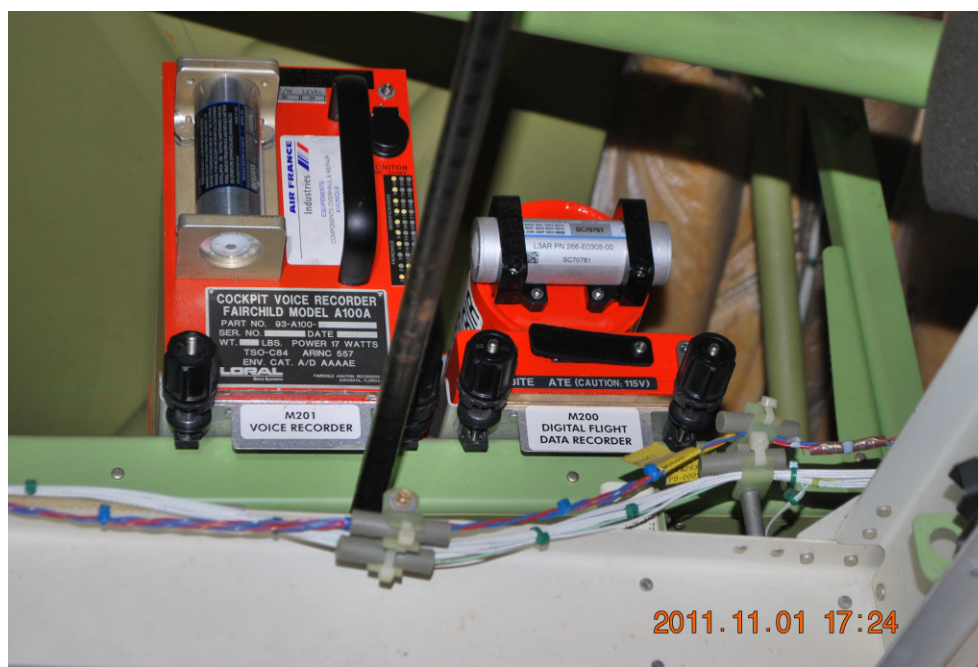
Photo 6. On-board recorders (FDR and CVR) of SP-LPC airplane.
