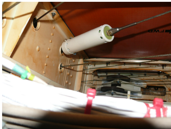
Photo 16. Load Limiter of the main left alternate landing gear extension system.
