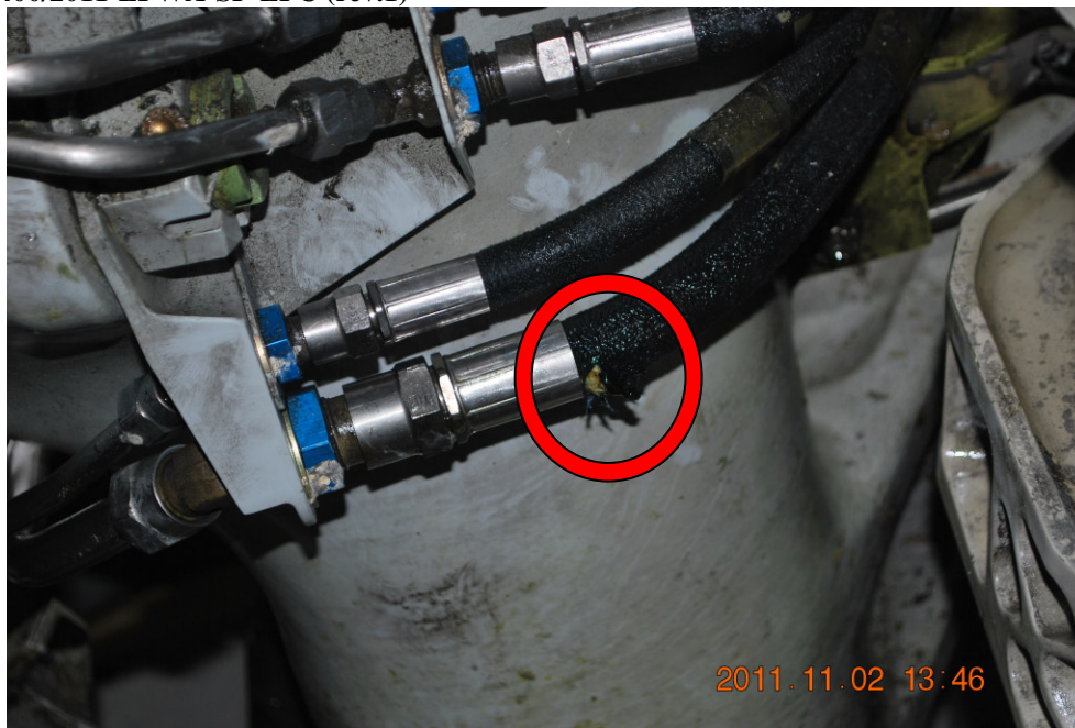
Photo 8. Damaged hydraulic hose of the right main landing gear of SP-LPC airplane.
